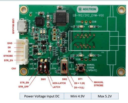
The two configuration switches S1 and S2 are present to match switch type. Do not change it.
